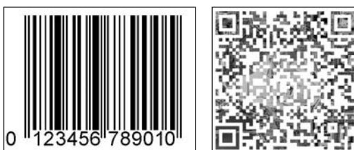
Picture 2: One-dimensional bar code (left) and two-dimensional bar code (right)
